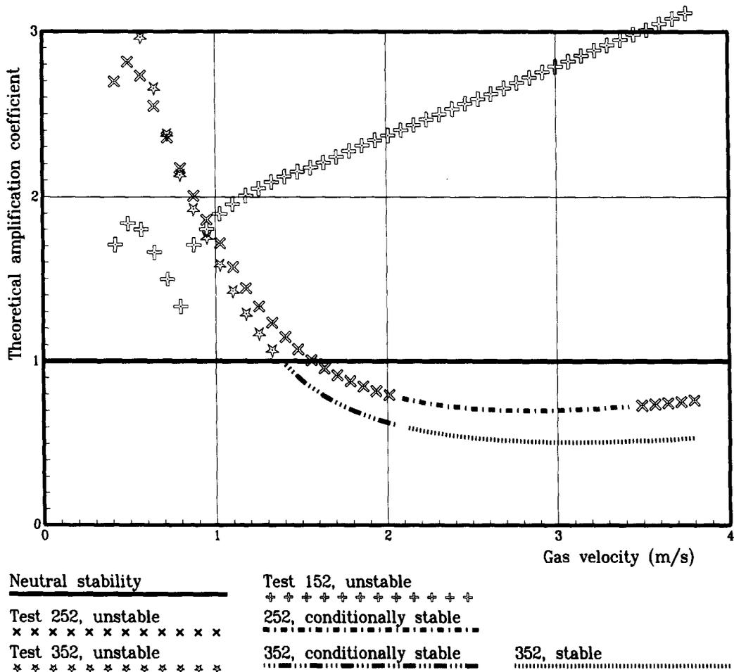
Figure 7. Effect of inertia and friction in the liquid suction pipe on airlift stability.
