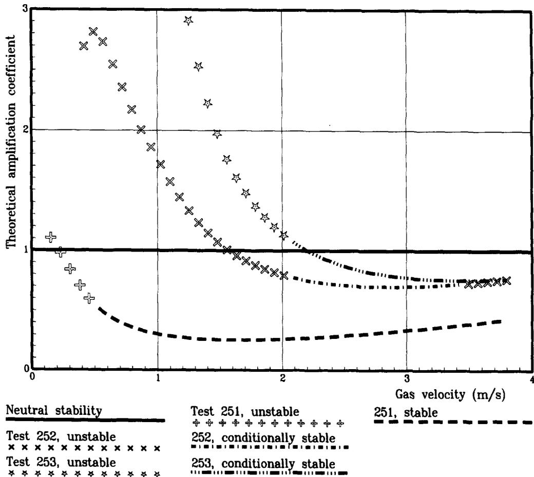
Figure 9. Effect of gas pipe volume on airlift stability.
