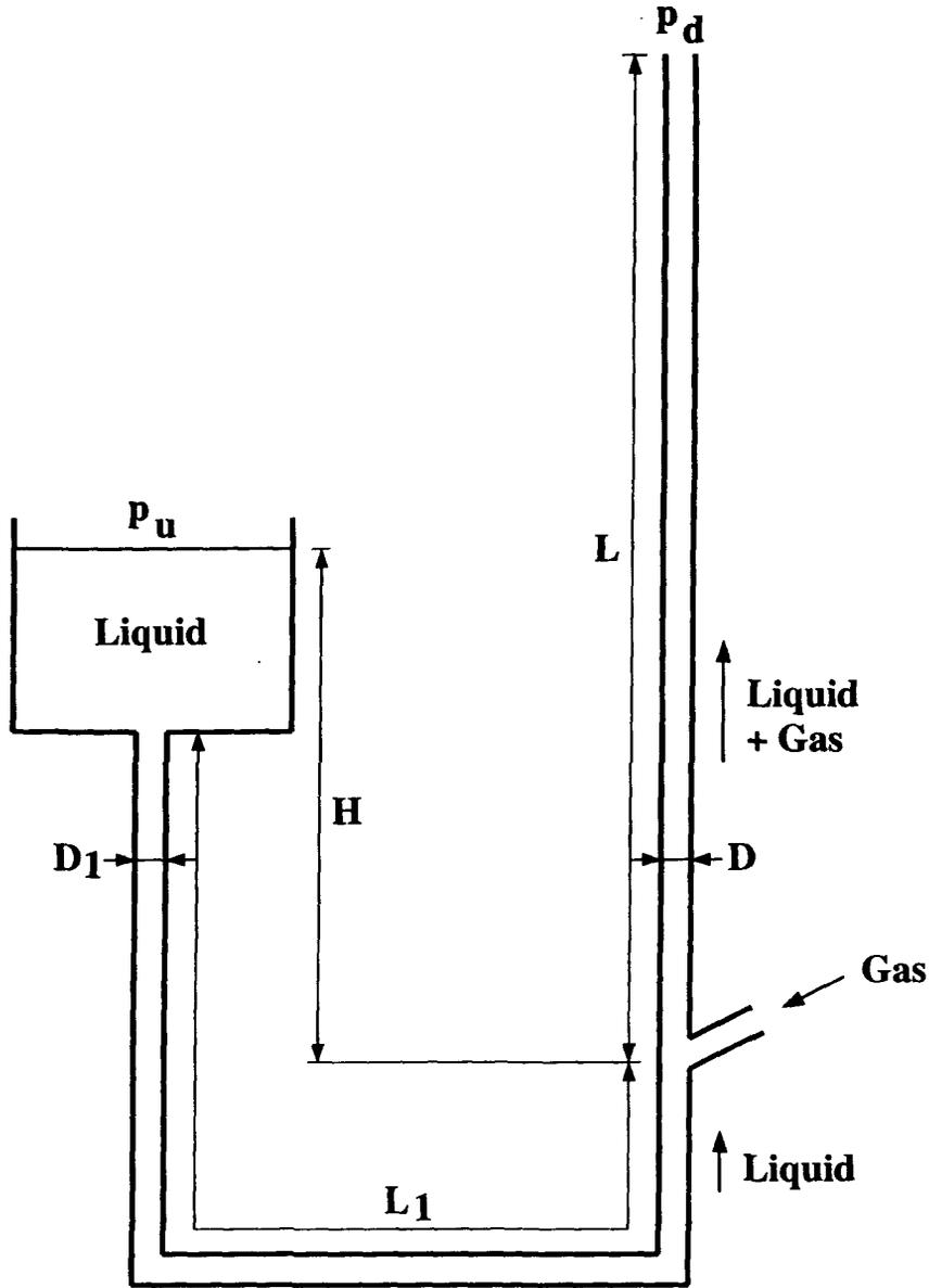
Figure 1. Typical airlift geometry.  $D$ ,  $D_1$ : internal diameters of the riser and of the liquid suction pipe, respectively;  $p_u$ ,  $p_d$ : upstream and downstream pressure;  $S$ : submergence, defined as  $H/L$ .
