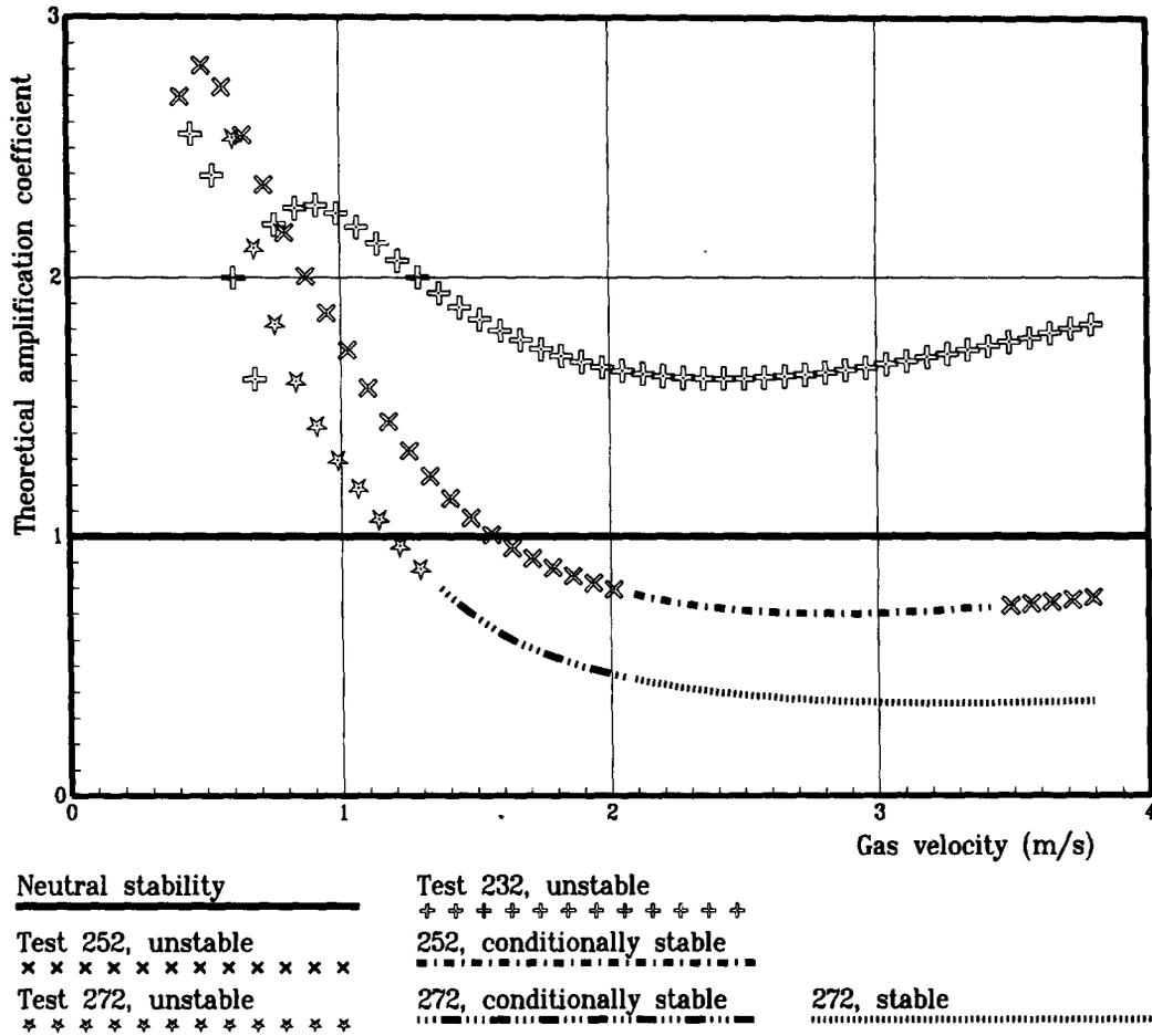
Figure 8. Effect of submergence on airlift stability.
